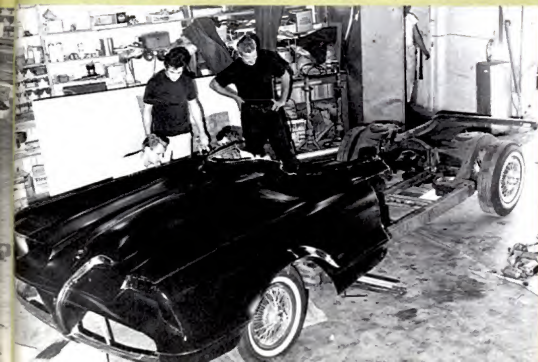
Constructing the Batmobile, fiberglass front end being installed on the frame.
